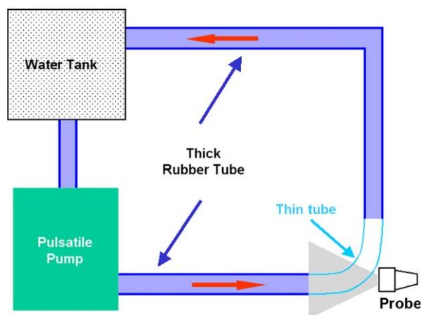
**Figure 1** Diagram of the flow phantom. The imaging window was selected towards the junction of the thick and thin tube.
